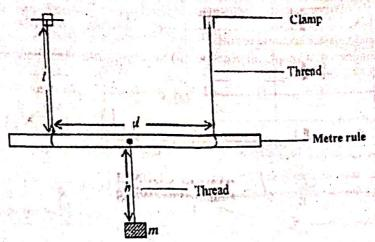
You are provided with a set of masses, two metre rules, a piece of thread, two retort stands and clamps, a stop watch, split corks and a weighing balance.
